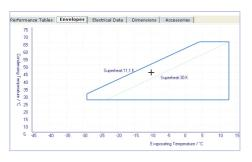
In the envelope tab the cross-hair shows the actual operating point specified on the first page either by Standard Operating Conditions or the conditions specified by the user.
