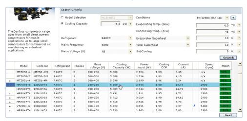
If you click on the "+" symbol to the left of any of the compressor models, the list of possibilities for that particular model is shown.
